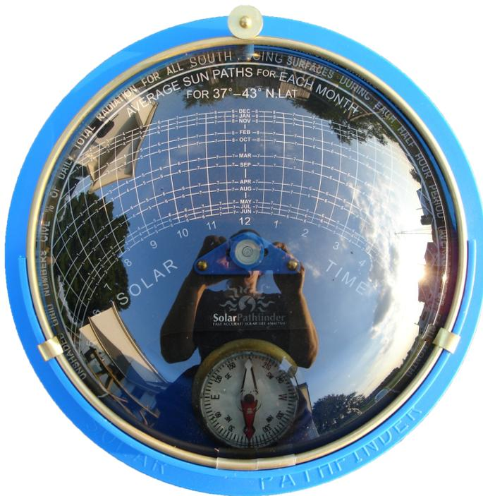
The Solar Pathfinder™ uses a highly polished, transparent, convex plastic dome to give a panoramic view of the entire site. All the trees, buildings or other obstacles to the sun are plainly visible as reflections on the surface of the dome. The sunpath diagram can be seen through the transparent dome at the same time.
