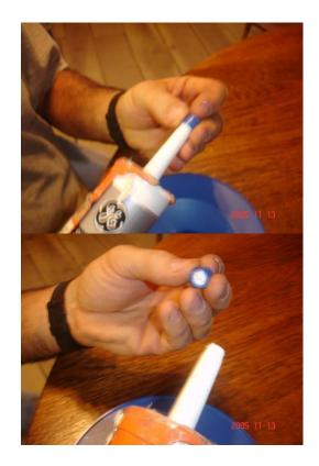
5. Using the superglue, leave a small bead of glue around the bottom of the sleeve.
