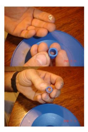
Fill (don't overfill!) the bottom of the sleeve with the white caulk. (This white caulk will give the level its contrasting color so that it is easier to read.)
