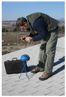
When viewing the Pathfinder, you are looking for two things at the same time. First a reflective, panoramic view of the site will be seen **on** the dome. Simultaneously, the sunpath diagram will be seen **through** the dome. Where the reflected objects on the dome intersect the sunpaths shown through the dome, the site will be shaded at the time indicated on the diagram.
