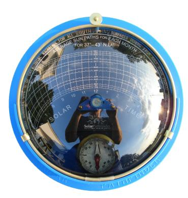
The Solar Pathfinder<sup>™</sup> uses a highly polished, transparent, convex plastic dome to give a panoramic view of the entire site. All the trees, buildings or other obstacles to the sun are plainly visible as reflections on the surface of the dome. The sunpath diagram can be seen through the transparent dome at the same time.
